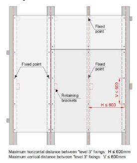
Image 18 – Example of cladding with Silbonit fiber-cement panels. The retaining bracket shown in red should be as close as possible to the fixed point of the panel.
