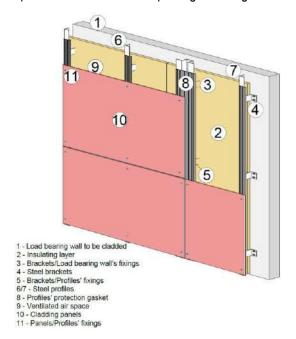
Image 13 - Example of a ventilated facade package with a steel subframe, mounted on the load-bearing wall
