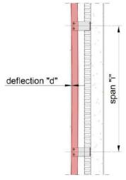
Image 7 – The maximum deflection of the battens/profiles between two brackets d<sub>max</sub> must be ≤ 1/200 for the span between the brackets "i"
