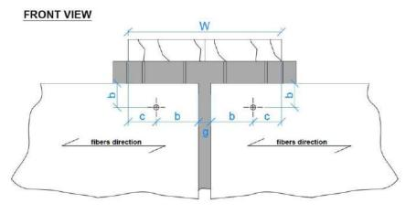
Image 11 - Geometrical specifications of the cladding required to determine the width of the wooden beams of the subframe
