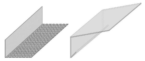
Image 5– Example of standard sections available for metal grilles and flashings used to protect the ventilated cavity.
