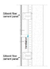
Image 26 – Example of a vertical section of the ventilated facade package along a horizontal joint between panels. Wooden subframe and Silbonit fiber-cement flat-panel cladding.
