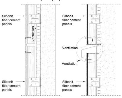
Image 16 – Example of a continuous and partitioned ventilated cavity on a wooden subframe. The flashings used to partition the air barrier must never compromise the free flow of air. The layer of insulation material is optional.
