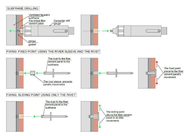
Image 21 – Example of steps to fix Silbonit fiber-cement panels. The panels are pre-drilled with holes that all have the same diameter of 9.5 mm. The example shows how the diameters of the holes for the fixed points are reduced using suitable metal bushings.
