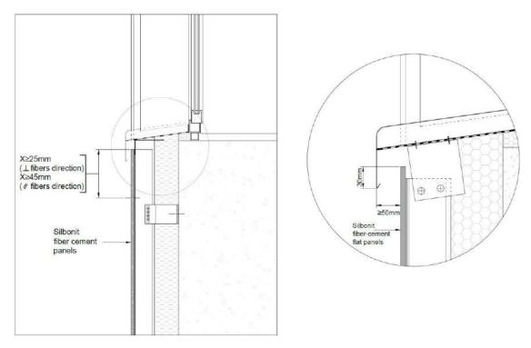
Image 34 – Example of vertical section of a ventilated facade along a window. Aluminum subframe.
