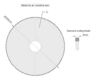
Image 45 – Example of a blade used to cut the panels at the Società Italiana Lastre SpA plant
